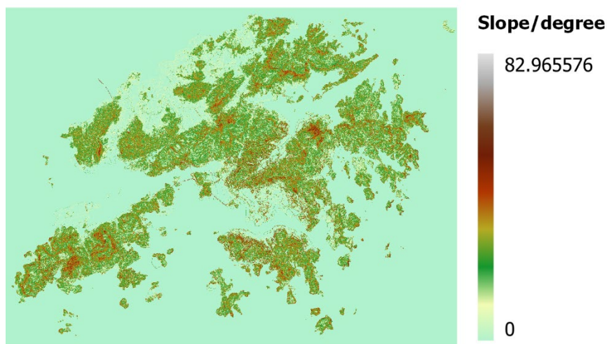
Figure 12. Slope calculation with the DTM data using QGIS with z factor of 1.0.
